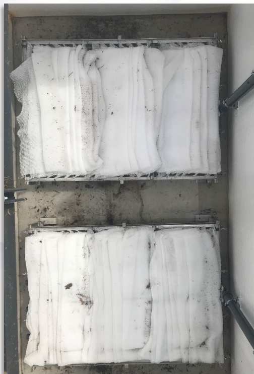
Bottom Right: WavTex modules in tank as it is being filled. The buoyant EnTextile sheets are beginning to stand.
