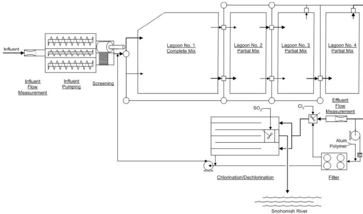
**Figure 1. Wastewater flows by gravity from the headworks to the complete-mix 10 MG surface aerated lagoon, then through a series of three 3.5 MG partial-mix lagoons, before passing through the tertiary filter and disinfection system (McKone, 2012).**
