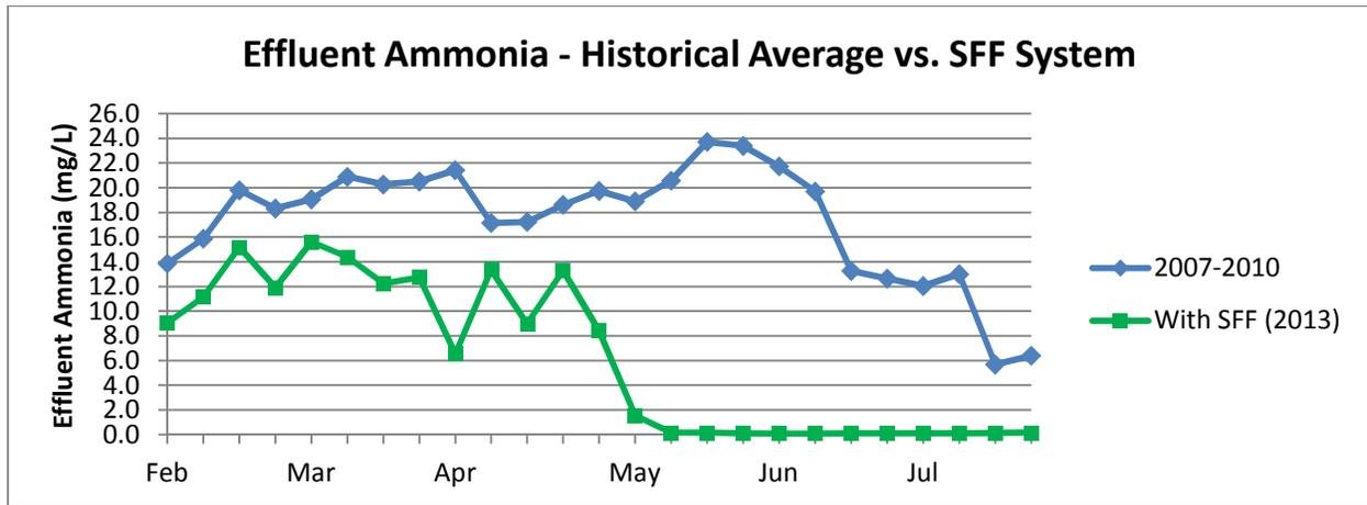
**Figure 9. Effluent ammonia concentrations with the submerged fixed-film system fell below required levels (2.6 mg/L) well in advance of the permit’s effective date.**
