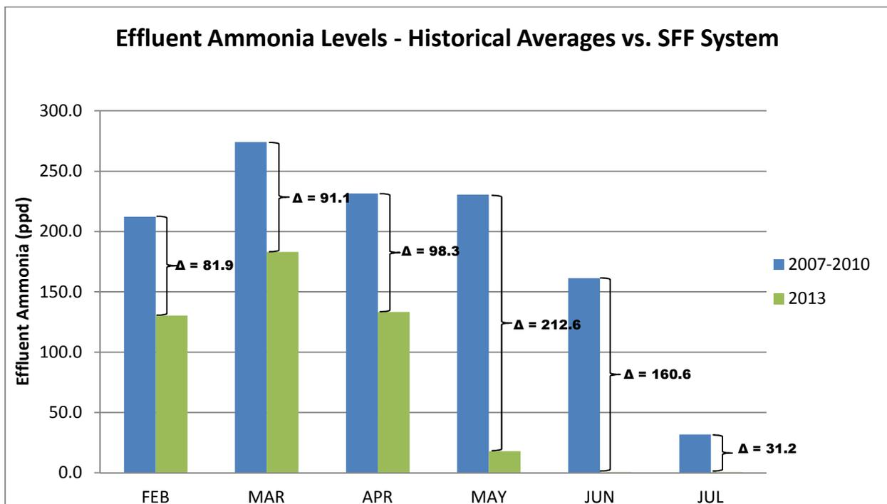
**Figure 8. Comparison of effluent ammonia levels. In May 2012, the plant achieved an effluent ammonia load that was over 200 ppd less than what was typically expected.**
