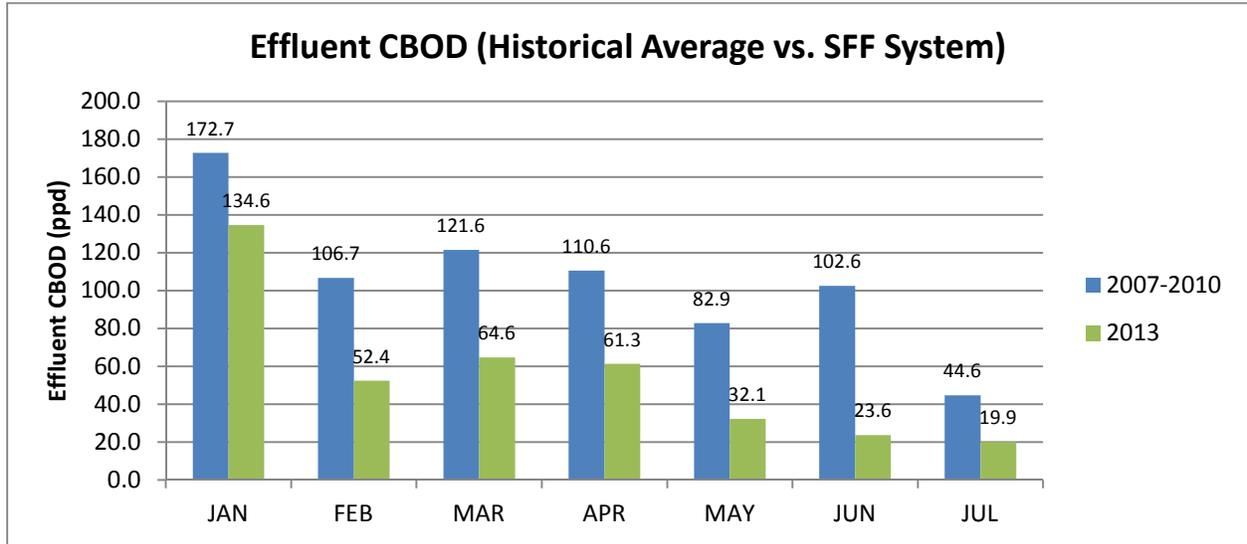
**Figure 6. Comparison of 2013 (YTD) effluent CBOD<sub>5</sub> levels to monthly averages from 2007-2010.**
