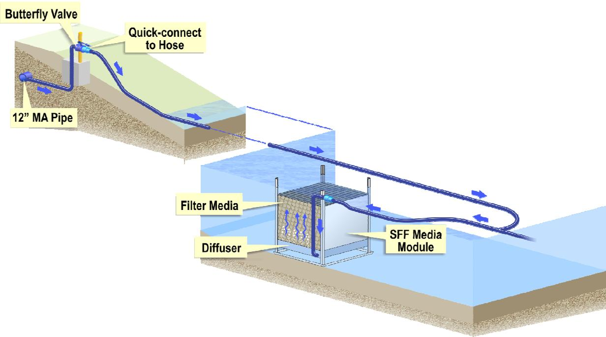
**Figure 5. Each pair of SFF media modules receives air through a 3” air line extending from the lagoon shore. Air flow is controlled by an electrically actuated butterfly valve. (Schuller & Giese, 2012)**
