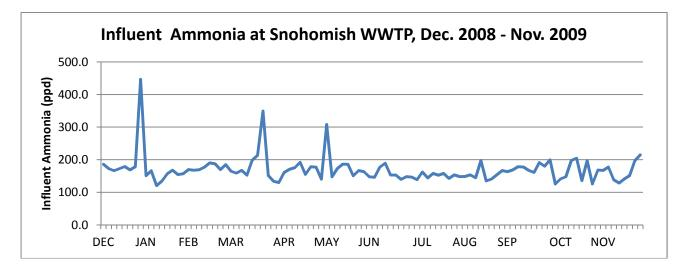
Figure 7. Influent ammonia loading at Snohomish WWTP over a one year period.
