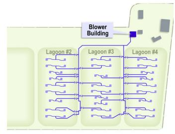
Figure 4. Plan view of the submerged fixed-film system. Modules closest to the surface aerators were placed nearer the edge of the lagoons. (Schuller & Giese, 2012)
