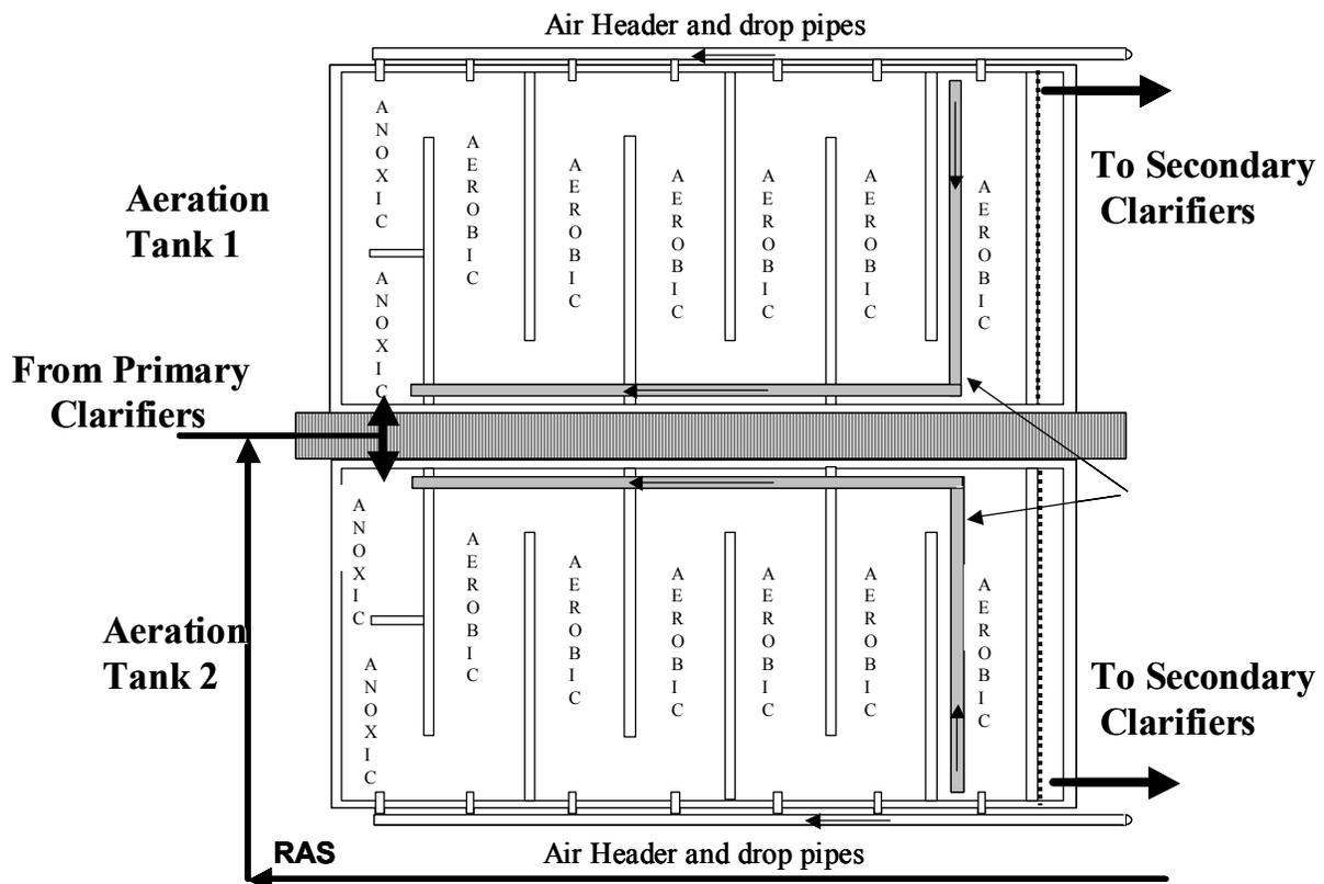
Because of the volume required in each basin for anoxic zones to achieve the degradation of nitrate, aerobic volume was effectively removed from the aeration basins. This volume reduced
