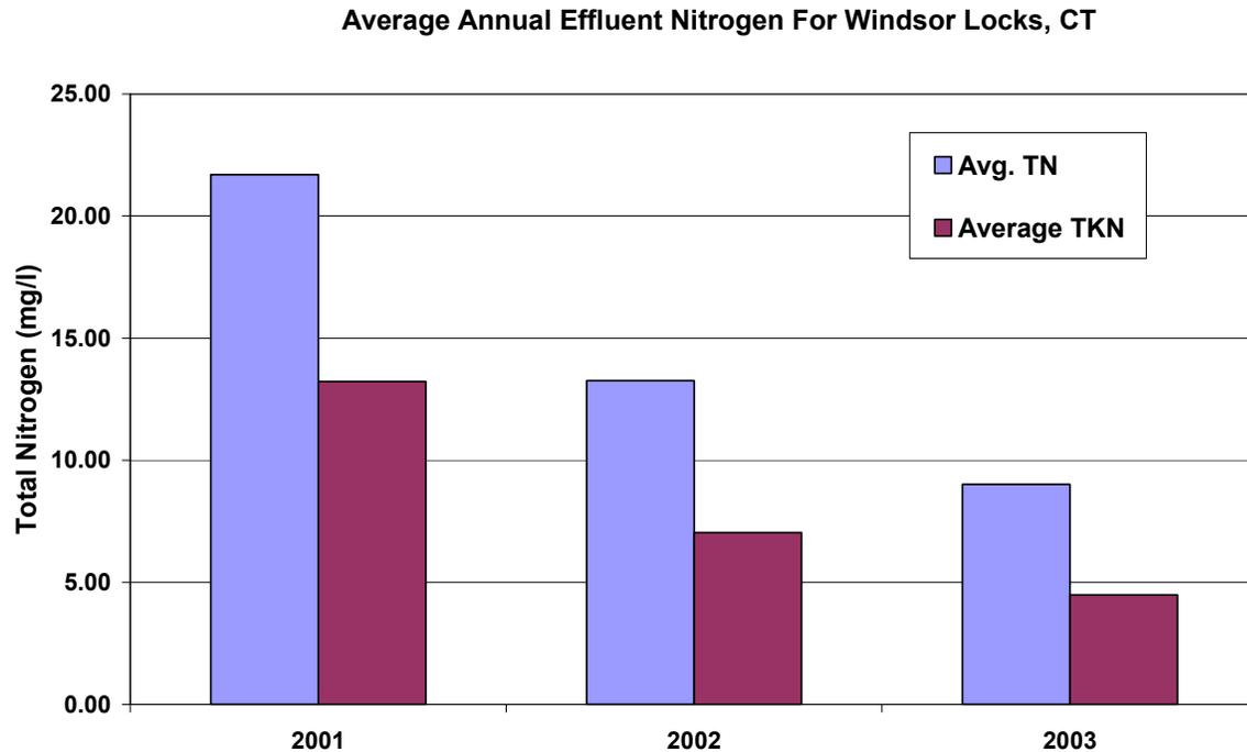
Additional benefits the plant has seen from the IFAS upgrade include better SVI test results and improved recovery from shock loads and plant upsets. This is attributed to the fixed-film component of the system, which traditionally has better sludge characteristics and is more able to handle toxic shock loads.
