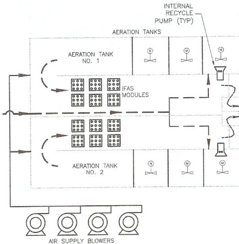
Figure 1 – New Process Flow Diagram – 25% Anoxic Volume
