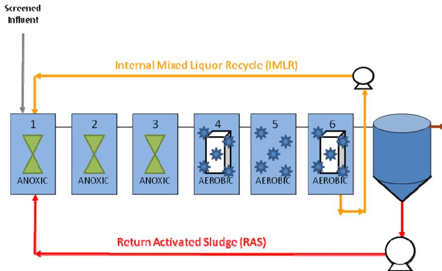
Figure 4 – Pilot Plant Flow Diagram
