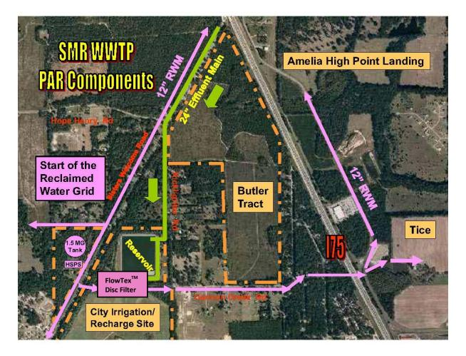
Figure 2. Lake City Public Access Reuse (PAR) Components.
